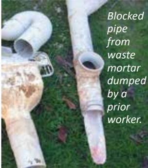
*Blocked pipe from waste mortar dumped by a prior worker.*
