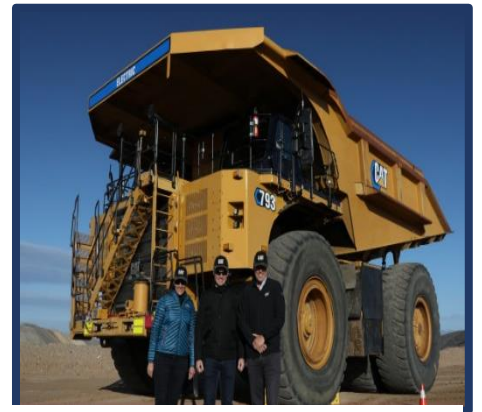
Australia's largest miner, BHP, is testing monster electric mining trucks in order to reduce fossil fuel use and carbon emissions
