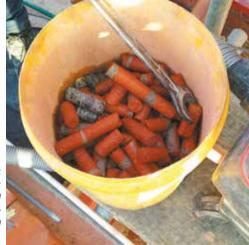
Sections of the cores of brick and mortar that were drilled out.
